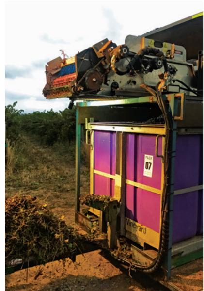
these units have a three to six percent waste stream. They are limited to the volume they can handle and the maximum capacity is 15 tonne per hour and at this level huge maceration occurs. For the world to effectively change to all new harvesters with inbuilt cleaning systems would take years. In Australia alone at the current rate of harvester sales it would take over 40 years and a massive amount of money.
